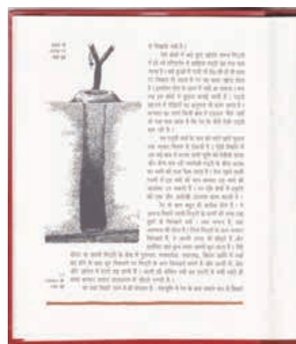
Figure 7. Diagram showing a kui going down to gypsum layer
